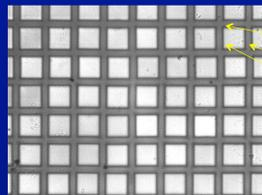
Optic plane is made from an array of slumped glass plates, each typically 4 cm x 4 cm, of 1 mm thickness.
