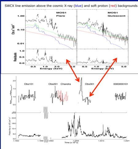
(Top) XMM EPIC X-ray spectra from flaring portion of light curve of diffuse emission (middle) from XMM (black) and Chandra (red). (Bottom) ACE solar wind proton flux (Carter, Sembay & Read 2010)
