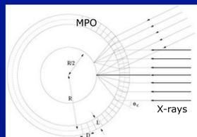
Principle of Lobster-eye optics. Parallel rays are brought to a focus at half the radius of curvature of the optic plane.
