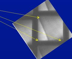
Plates have square channels typically 20 μm in width with a wall thickness of 6 μm (open area is ~ 60%)
