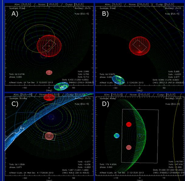
Example snapshots of the simulator FOV. Red and pink spheres represent North and South Cusps. Green represents the magnetosheath. Earth is the blue sphere. Sun avoidance region is in yellow.
