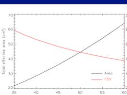
Optic design involves a trade-off between focal length, effective area and FOV for a given optic size. Here these parameters are shown for a 30 cm x 30 cm optic.
