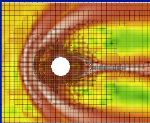
2-D cut of an MHD simulation of the plasma density around the Earth generated by the GUMICS-4 code (see Janhunen et al. 2012)
