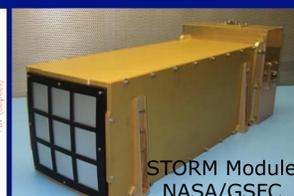
A prototype imager using one MPO (central facet) has been built by NASA/GSFC and flown on a sounding rocket experiment (Thomas, N. E. et al. 2013)
