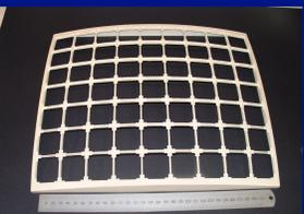
FOV is built up by placing required number of plates in a holder. e.g. 30 cm optic with a focal length of 37.5 cm has a 23° FOV. Typical optic mass is ~ 1 kg
