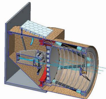
**Figure:** Telescope design used to study the feasibility of the mass payload assumptions.
