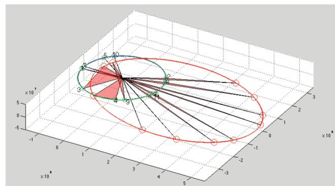
**Figure:** Orbit of asteroid Oljato exemplifying how the JPL small body data base was used to find suitable asteroids which could be tracked with a 30 cm telescope from L2 during a mission flown between 2014 and 2020. The visibility of the asteroid is shown in the next figure.
