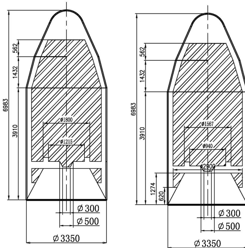
**LM-2D fairing static envelope with 1194 (left) and 937 (right) interfaces**
