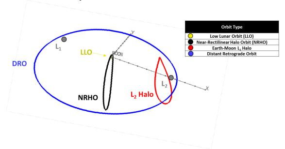
Figure 1 Orbit types reviewed for the Deep Space Gateway. Of those reviewed Near Rectilinear Halo Orbits and Earth-Moon L2 Halo orbits were found to be technically favourable.
