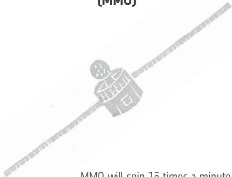
MMO will spin 15 times a minute once it is orbiting Mercury to help distribute the Sun's heat
