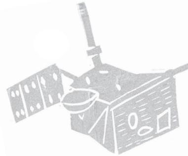
The MPO has a large 3.7m wide radiator to carry away heat generated by the spacecraft, as well as heat coming from the Sun and Mercury
