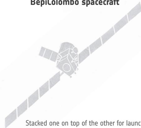
Stacked one on top of the other for launch, the composite spacecraft is about 6 m high
