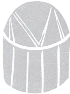
The sunshield gives thermal protection to the Mercury Magnetospheric Orbiter during the cruise to Mercury
